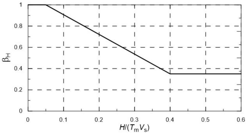
H slope height or height of retaining structure in contact with the soil  $V_{\rm S}$  shear wave velocity
