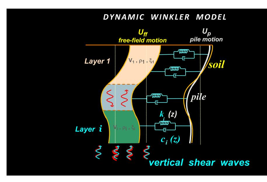
(4) With Winkler modelling, ground should be discretised into horizontal layers. Onedimensional ground response analysis should be conducted to obtain the time-histories of displacement at each layer. These displacements should be imposed at the supports of the lateral springs-and-dashpots.
