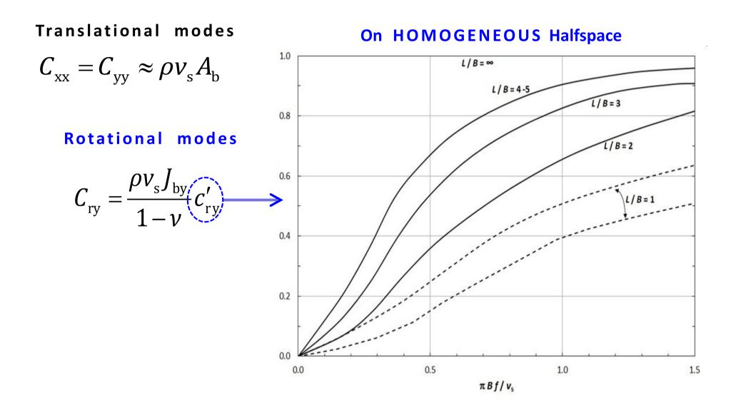
(4) Frequency-independent stiffness <u>may</u> be assigned to each spring, corresponding to the period of the fundamental mode, accounting for SSI in the considered direction. If this period is difficult to determine reliably, the <u>static stiffnesses</u> may be used instead.
