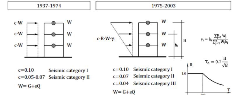
Figure 2. Seismic load definition pre- (left) and post-1975 (right).
