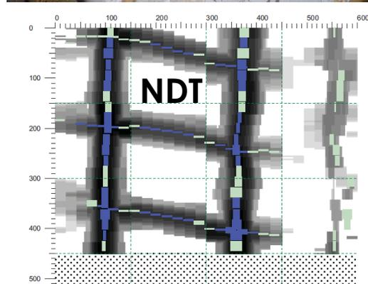
Bars in the top layer are not of the same type: TOR bars and regular deformed bars. This cannot be detected with non destructive techniques.
