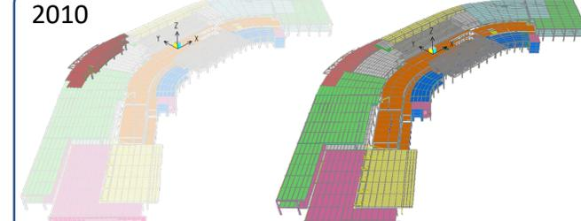
Airport terminal built starting in RC (NATO military airport, ACI code from the time) and ending with structural steel. Almost each addition was designed and built according to a different code...
