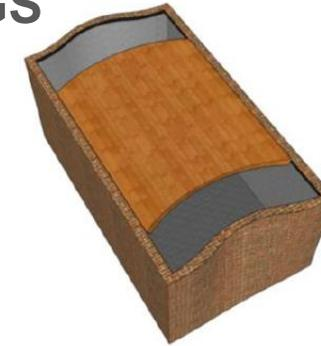
Displacement incompatibility between diaphragm and URM end walls.
