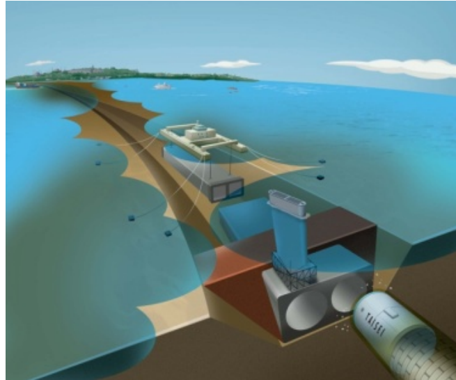
Figure 4. Conceptual image of tunnel construction and connection between immersed and TBM tunnels
